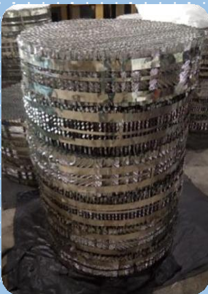
Distillation Column Packing
